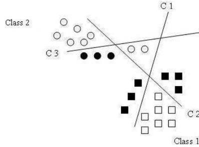
**Figure 1.** Aggregation of classifiers using a voting strategy. Bold patterns are misclassified by a single hyperplane but not by the combination.
